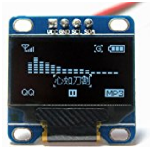
Figure 2: Small break-out-board SSD1306 128x64 Bit OLED Display
